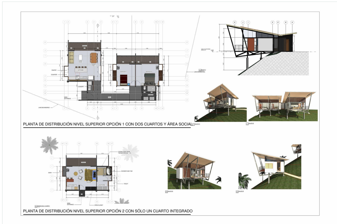
Figure 8 — Proposed, not built. Option 1: two bedrooms with a social area. Option 2: a single integrated room with an ocean view from the bathroom. Section and 3D views at right. One sheet of the plan set, shown as a sample of the drawing standard.
